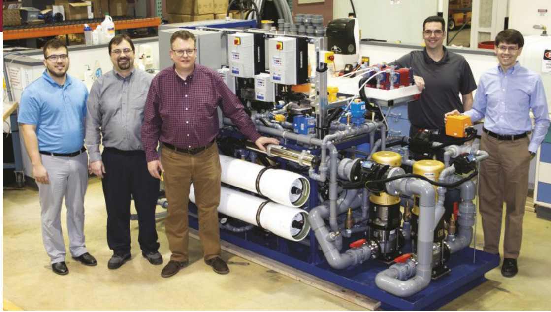
EVC’s Twin Ultra Greywater Recycling System was developed by a team of engineers including (left to right) Jorge Dias, Mark Pitterle, Brian Ott, Brian Gaston and Jeff Yanuck.
